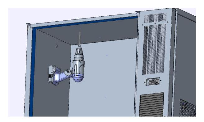
4. Place inserts and screw with screws A3.9x19 A2. White rods of bottom, upper and front insert has to be inline.
